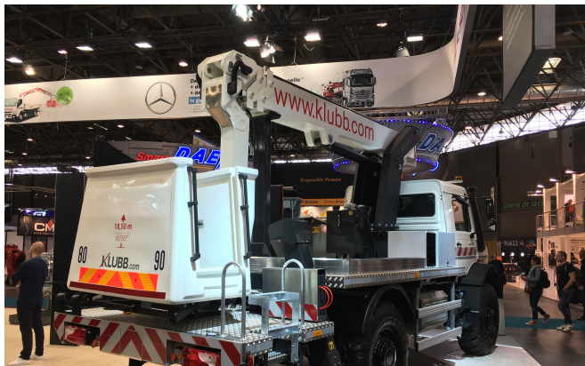
Xtenso3 on Unimog - 18,5m working height
