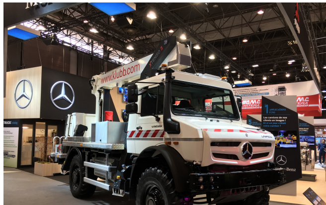
Xtenso3 on Unimog - 18,5m working height
